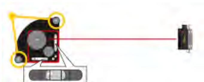
Rotate laser transmitter 180° and level the laser transmitter.
