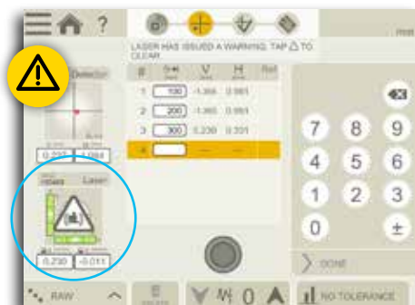
The built-in sensors warn on the display on events which can affect the measurement reliability.
